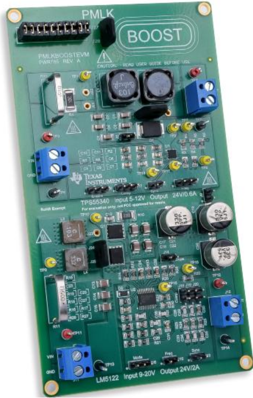
Figure 2. BOOST converters for the lab demonstrations.
