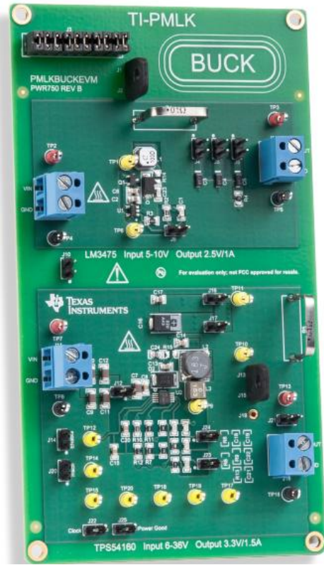
Figure 1: BUCK converters for the lab demonstrations.
